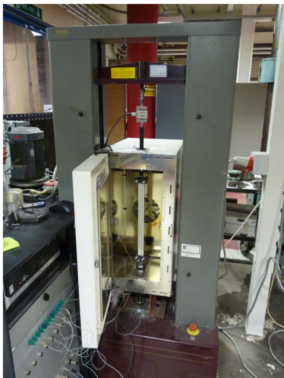
Figure 2. Experimental setup for heat-activated stress relaxation tests. [Color figure can be viewed in the online issue, which is available at wileyonlinelibrary.com .]
