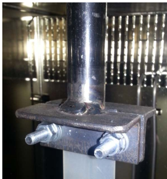
Figure 1. Grip used to hold ends of test specimens. [Color figure can be viewed in the online issue, which is available at wileyonlinelibrary.com .]
