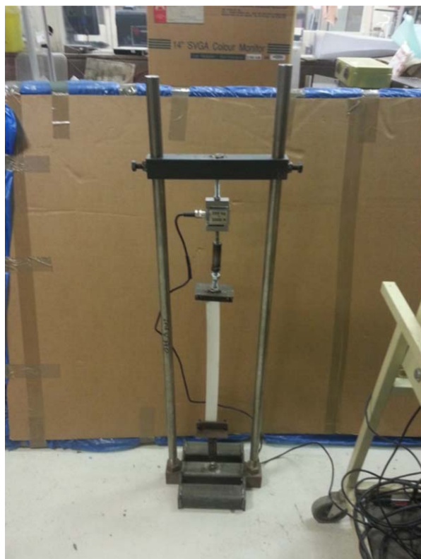
Figure 6. Experimental setup for manually applied stress relaxation tests. [Color figure can be viewed in the online issue, which is available at wileyonlinelibrary.com .]
